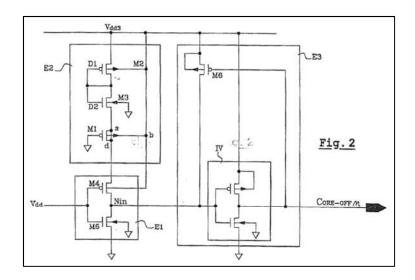
(Appx1264.) The detection device "comprises an output stage E3 following the input stage E1, to obtain the desired output levels for the inverse detection signal  $C_{ORE-OFFn}$ ." (Appx1270 ¶ 0037.)
