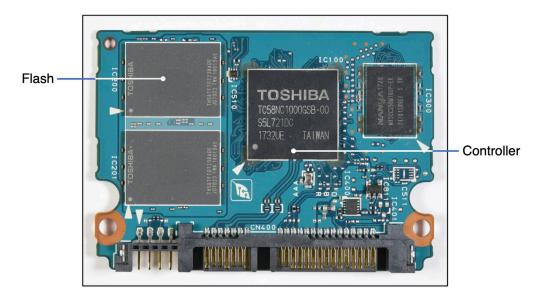
57. The Accused Products all contain a flash memory decoder comprising a decoding module configured to receive encoded data from flash memory. For example, on information and
