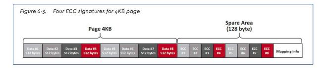
65. On information and belief, as part of the read-out of data from the flash memory, the encoded data (in the form of the stored data and ECC signature) is received by the decoding module, as described below in Western Digital's White Paper.<sup>20</sup>
