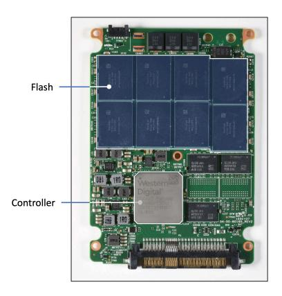
55. On information and belief, the controller in the WDS960G1D0D SSD includes a flash memory decoder and a decoding module configured to receive data with an ECC signature, such as that displayed below, taken from a Western Digital White Paper publication regarding its flash memory products, for a 4KB page flash with 8 ECC signatures (one for each 512 bytes of
