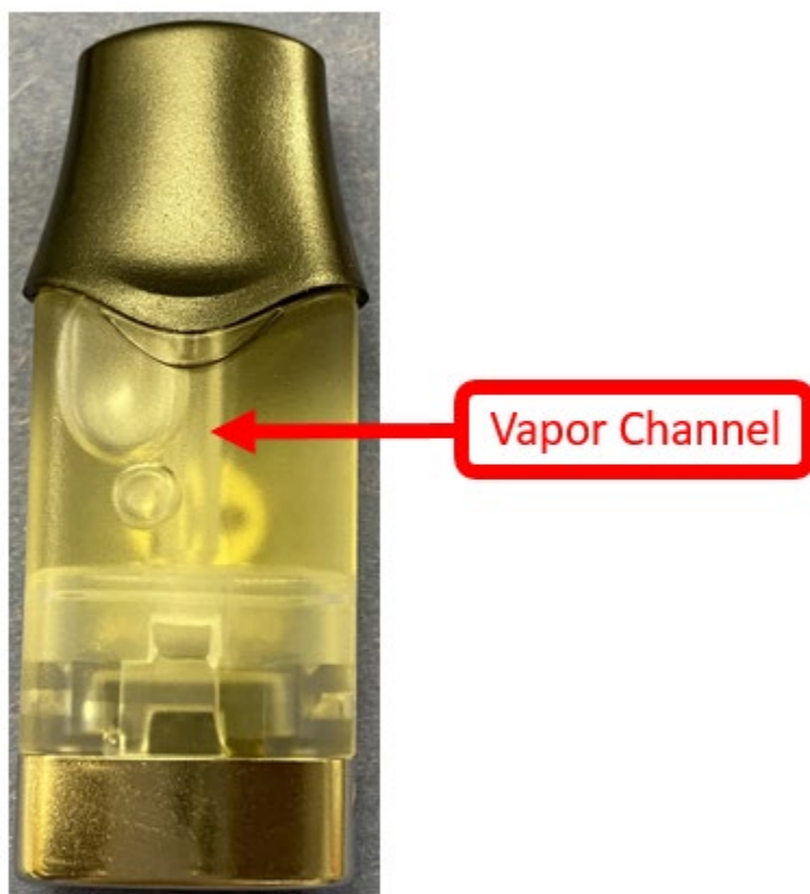
The Accused VUSE ALTO Products (Vapor Channel Shown)
