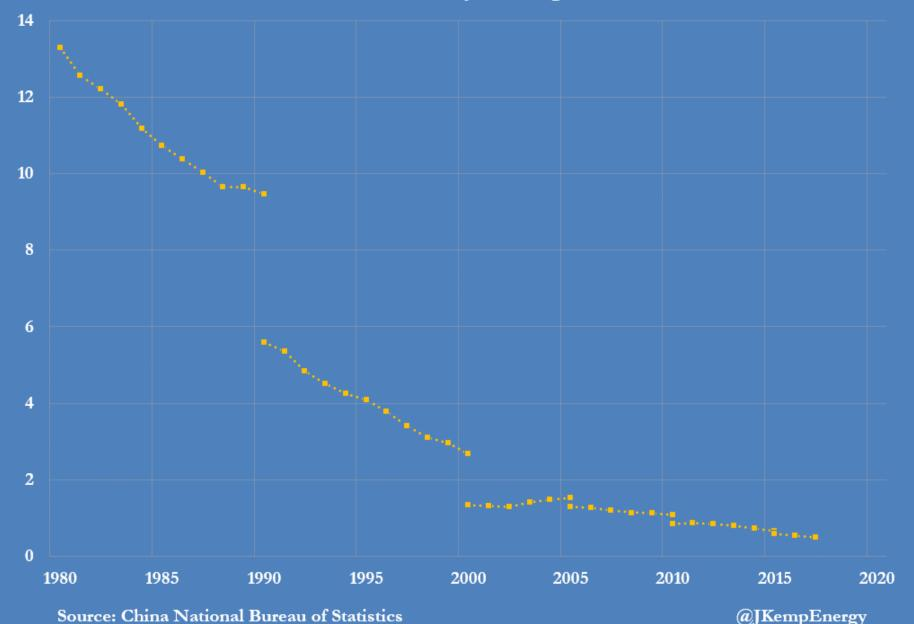
China energy efficiency - coal consumption / GDP ratio tonnes of standard coal equivalent per 10,000 yuan at constant prices *semi-logarithic scale*, discontinuities caused by rebasing of real GDP
